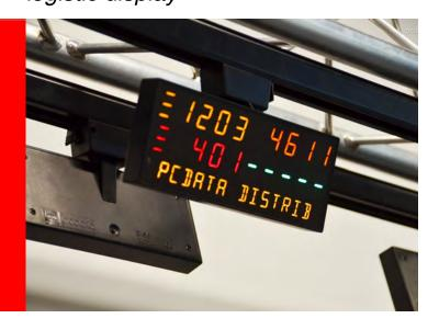
The DIS5 is Pcdata's 5-field logistic display. It can show all necessary information to warehouse personnel that are handling goods. It has a connector for electrical and mechanical connection to a standard conductor rail.
