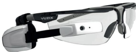
The Distrib AR module is based on Augmented Reality, with the use of wearable mobile technology (Smart Glasses). The solution offers similar high-performance, hands-free guided picking operation as with the standard Put & Pick to Light solution, however without the need for fixed structures and initial investment in hardware.
