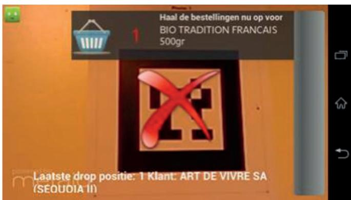
If the operator is looking at a location Marker, for which no product is needed, the App will show the operator that this location can be bypassed. The Smart Glass will also inform the operator of the location of the next drop; next to this the App also indicates the progress of the picking activity in a progress bar. In an environment with a number of locations next to each other, the operator can see up to 5 positions simultaneously, offering him the possibility to plan his next actions.
